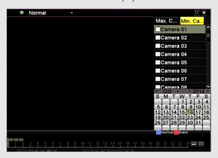
Press the PLAY button to move between Max.Ca, Min. Ca and Camera 1 using joystick (DS-1003KI) or arrow keys (remote control).
