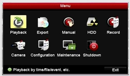
Use the joystick (DS-1003KI) or arrow keys (handheld remote control) to navigate to the Playback icon and press ENTER button to enter into the below playback screen:
