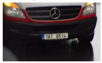
**Solution:** Not enough shutter speed of the camera. Should be reduced to 1/1000 or 1/2000 depending on vehicle speed and lighting.
