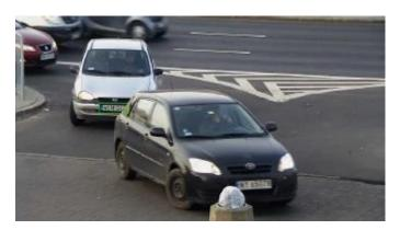
**Solution:** Notice how there is not enough focus for all frame. Car with a green frame will be decected, and other cars will not. Adjust the focus on the lens.
