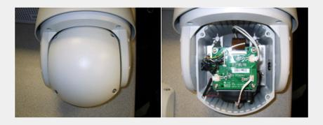
The Micro SD memory slot is located on the top of the camera module to the left of the ribbon cable as shown below:
