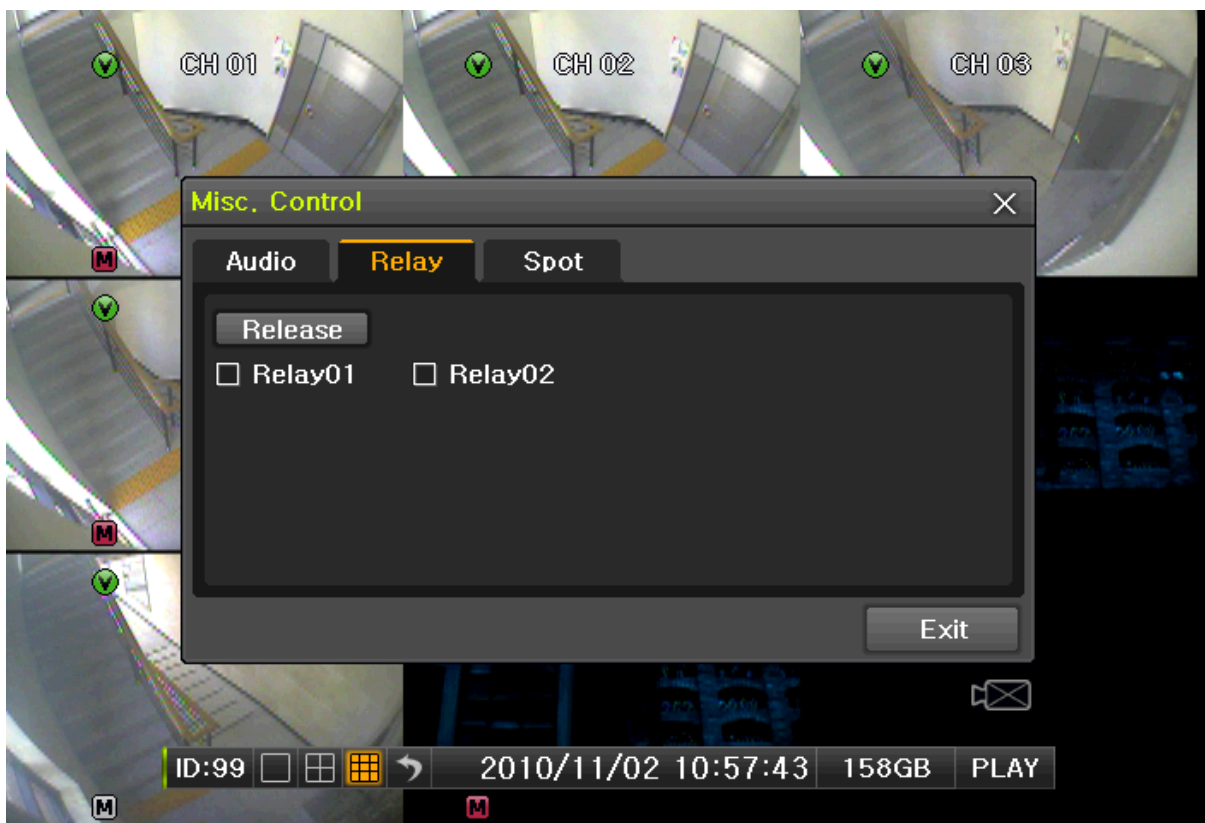
[Figure 5-14. Relay Control Window]
