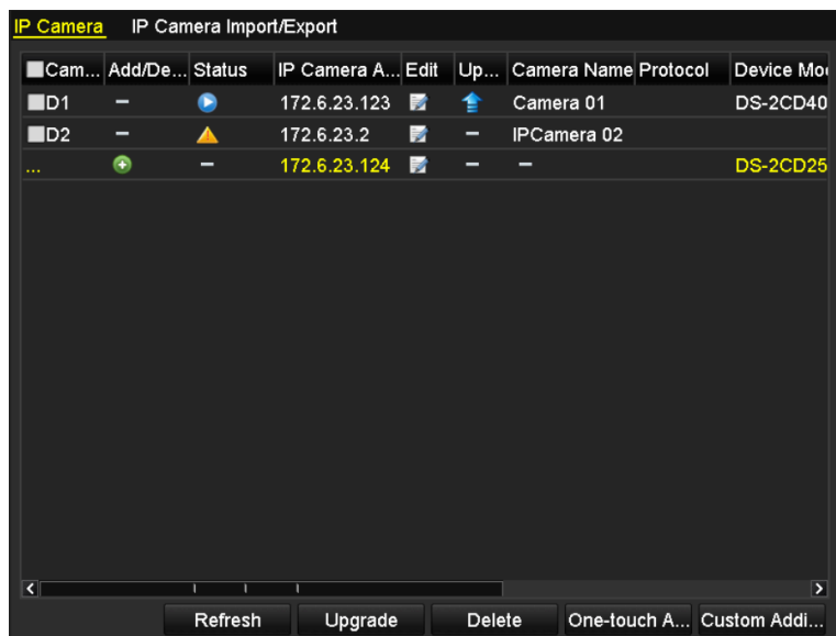
Figure 2. 16 IP Camera Management Interface
