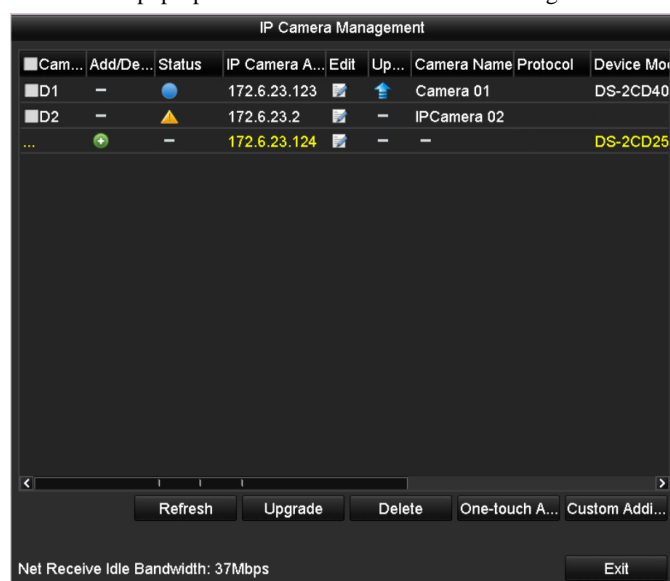
Figure 2. 13 Adding IP Camera Interface
