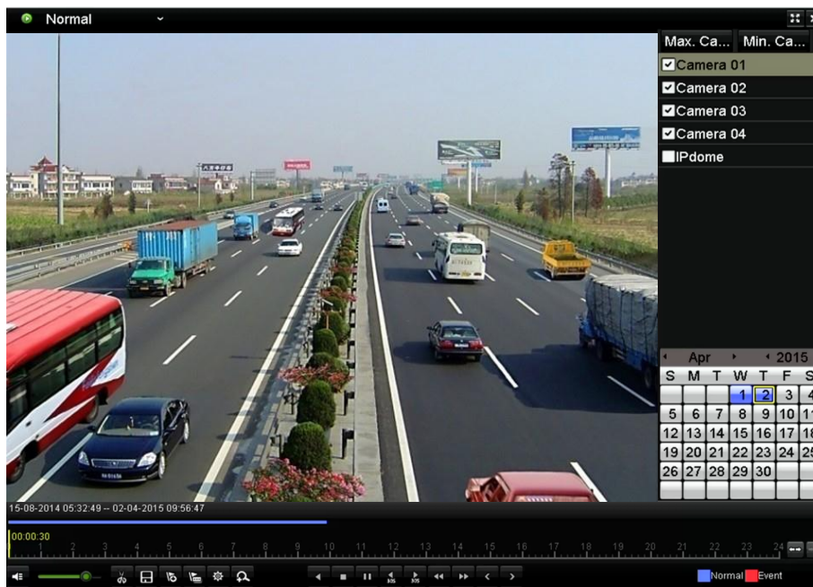
Figure 6.9 Interface of Playback by Time
