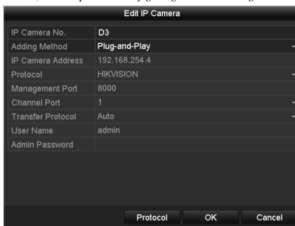
Figure 2. 24 Edit IP Camera Interface - Plug-and-Play
