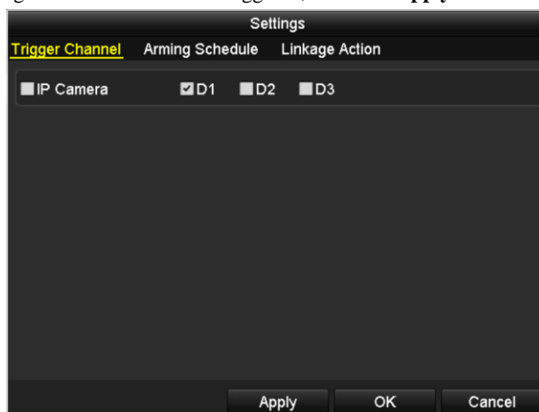
Figure 8.2 Set Trigger Camera of Motion Detection
