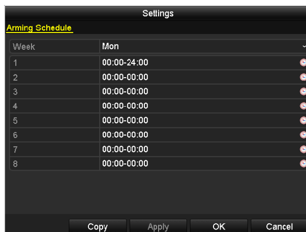
Figure 8.19 Set Arming Schedule of Alarm Output
