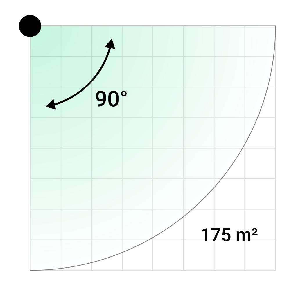
With the 90° horizontal viewing angle, MotionCam Outdoor (PhOD) Jeweller can cover up to 175 m² area.
