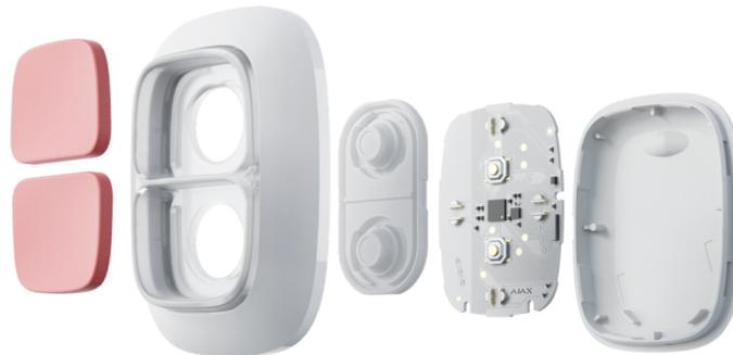
To activate the alarm, you must simultaneously press both buttons. They are stiff and parted by a plastic barrier. These measures eliminate false alarms when carrying DoubleButton in a pocket or bag.
