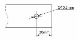
**Note:** When drilling new holes always ensure they are diametrically opposite each other so that the bolt can pass straight through.
