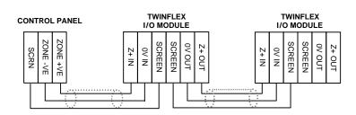
The Twinflex I/O Module can be mixed on the same zone as other types of Twinflex device (eg. Twinflex Multipoint Detectors). The above diagram shows how to make the zone positive, zone negative and screen connections between the control panel and Twinflex I/O Modules. Refer to the instruction leaflets supplied with other Twinflex devices for their equivalent wiring/terminal labelling details.
