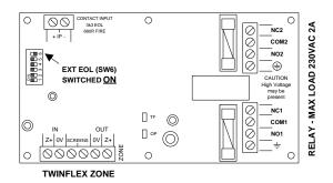
For use as a simple 'change-over' relay output, connect to relay contacts as above, **remembering to set the External EOL switch to ON**.
