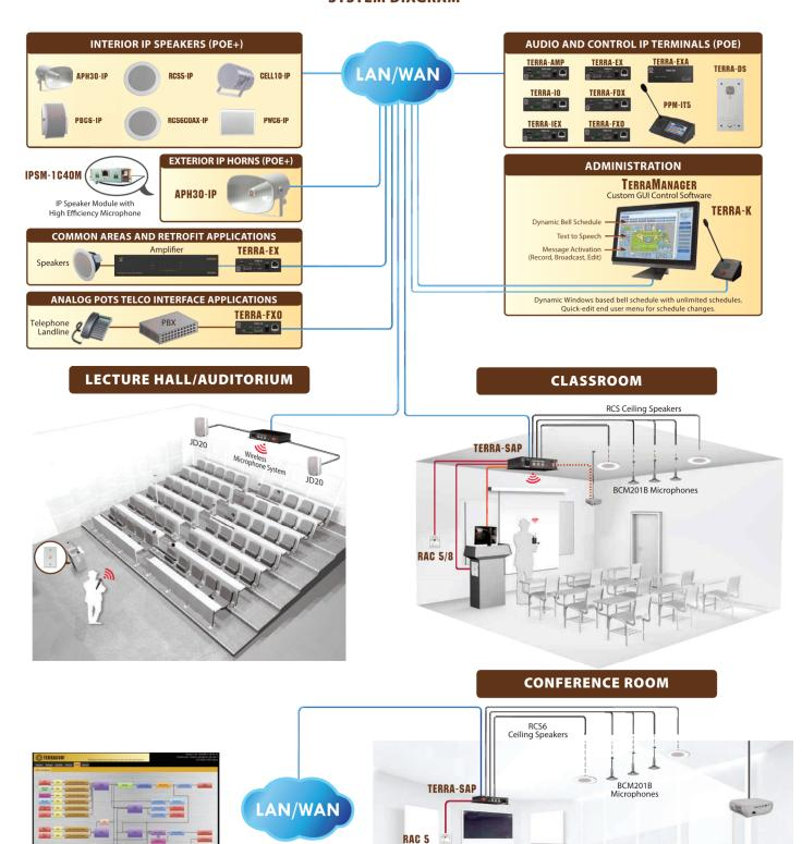
"Full DSP for advanced audio adjustments such as input muting priority management, EQ, Filters, Noise Suppression, AEC, Comp/Limiter, Feedback control, AGC and I/O level adjustments - all via HTML web browser programming"
