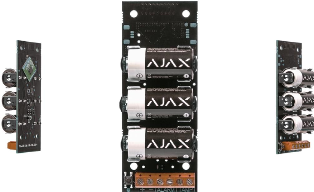
Wireless module for connection of outdoor motion detectors, IR barriers, liquid level detectors, and gas detectors, thermal relays and any third-party devices with wired output to the Ajax security system.
