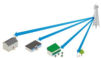
The NanoBeam 5AC Gen 2 used as a CPE device for each client in an airMAX PtMF network.
