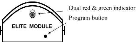
1. To enter program mode press and hold down the program button - the 'RED' indicator lights for 4 seconds then the 'GREEN' indicator sequences through the six 'selections'. **One** flash for the range, **two** for the pulse count. **Three**- LED monitor. **Four**- 'S' lux level. **Five** for CCTV mode and **six** to change the timer setting.
