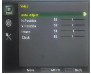
**AUTO ADJUST:** Perform an automatic configuration of the Phase, Clock,
