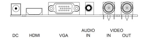
**XDC:** Only use the 12v DC power supply included with the monitor.
