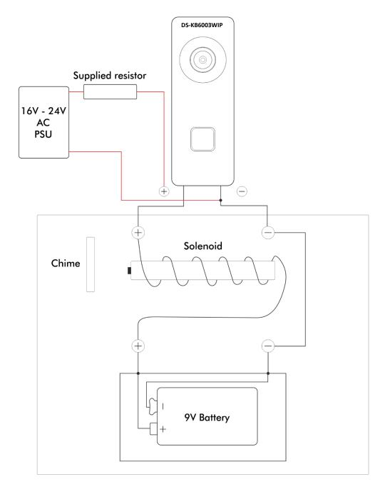
When powering the DS-KB6003WIP WiFi doorbell from a separate PSU as above it is important that the supplied resistor is wired in series with the PSU feed to act as a dampener, failure to do this could result in damage to the DS-KB6003WIP through over voltage. The chime circuit can be powered using a separate battery (ensure you select the appropriate model chime) and wired to the DS-KB6003WIP in parallel with the PSU as shown above.
