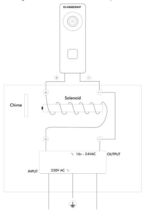
When using a mains powered chime to power your DS-KB6003WIP Wi-Fi doorbell it is important that the chime has an output voltage of between 16 to 24 volts AC feeding the solenoid and in turn the doorbell, if the chime output voltage is lower than 16 volts this will cause operational problems with the DS-KB6003WIP in particular its ability to connect to the cloud server and forward calls through to your mobile device.
