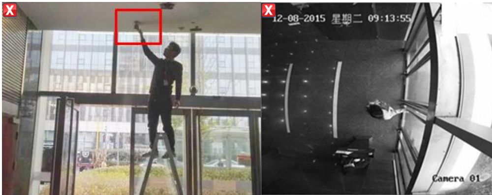
Passenger flow in horizontal direction (wrong)
