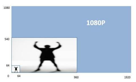
For example, the target in the picture below is too large to detect, the man almost covers the whole scene. We suggest adjusting the angle higher so that IP camera can start detecing from a longer distance.
