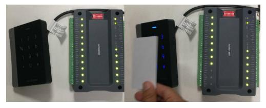
I give this card the permission of the first three floors, after swiping card, We can see the corresponding relay acted by these pictures $_{\circ}$
