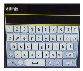
You can now move around the characters using the joystick and press the ENTER button to select a specific character, repeat this process until your login password is complete then move to the return icon (bottom right hand corner) and press the ENTER key to confirm password. Now you only need to move down to the OK icon and press ENTER to display menu GUI icons.
