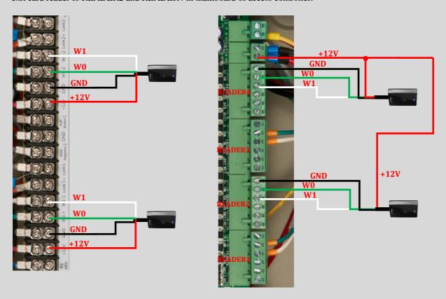
Note: We can also connect exit button to wiring distribution in access controller for exiting.
