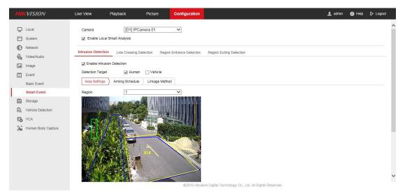
Please note NVR can support false alarm reduction for line crossing, intrusion detection, region entrance and region exit, but only two of them can be enabled simultaneously in the same channel when the **Local Smart Analysis** is enabled. If you don't tick 'Enable Local Smart Analysis', NVR would receive the alarm picture from IPC to filter false alarm (only work with Hikvision 4/5/7 line camera).
