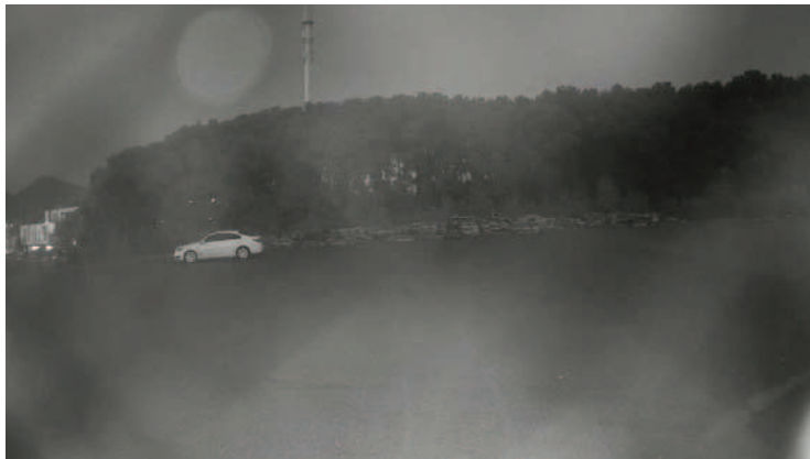
Figure 1 Image Dimness Caused by IR Reflection
