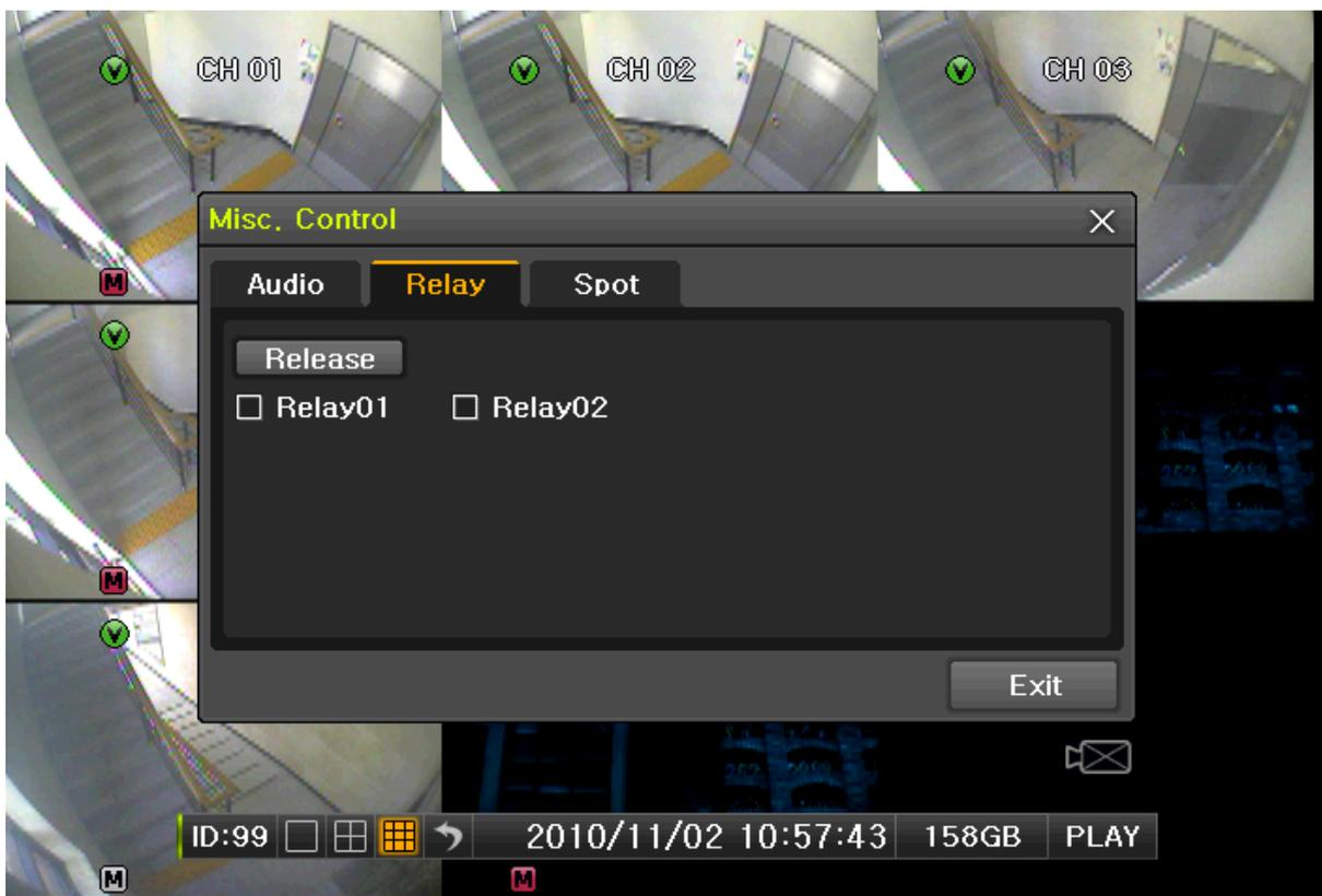
[Figure 5-14. Relay Control Window]
