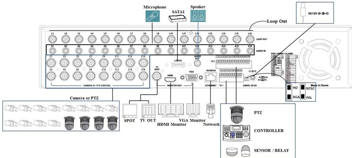
[Figure 2-3. MX-16DA Basic Connection and Device Connection]
