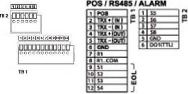
[Figure 2-8. MX-8DA Terminal Block and Description]
