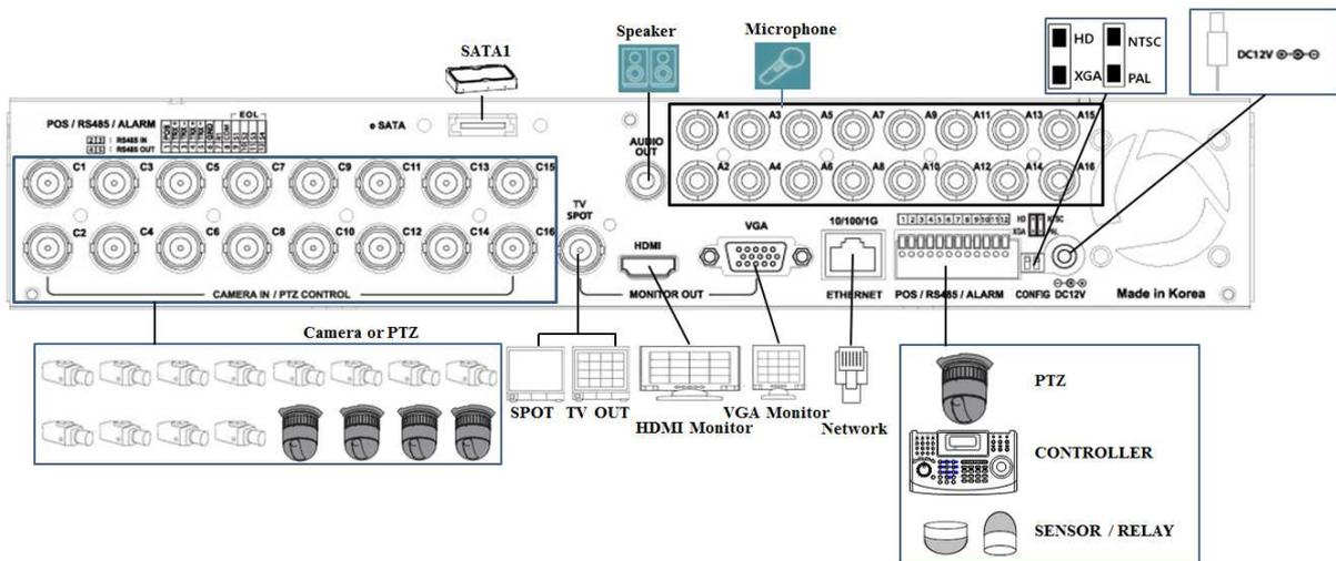
[Figure 2-6. MX-16A Basic Connection and Device Connection]
