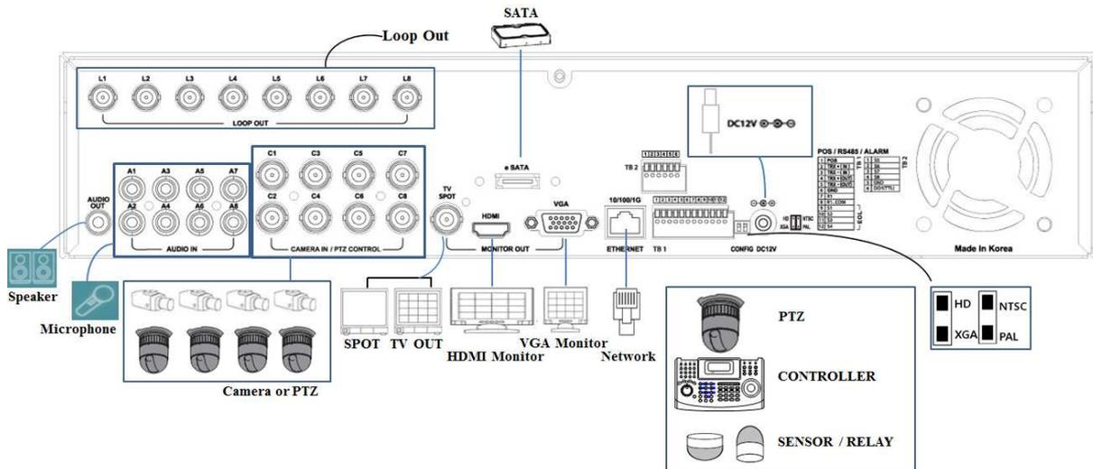
[Figure 2-2. MX-8DA Basic Connection and Device Connection]
