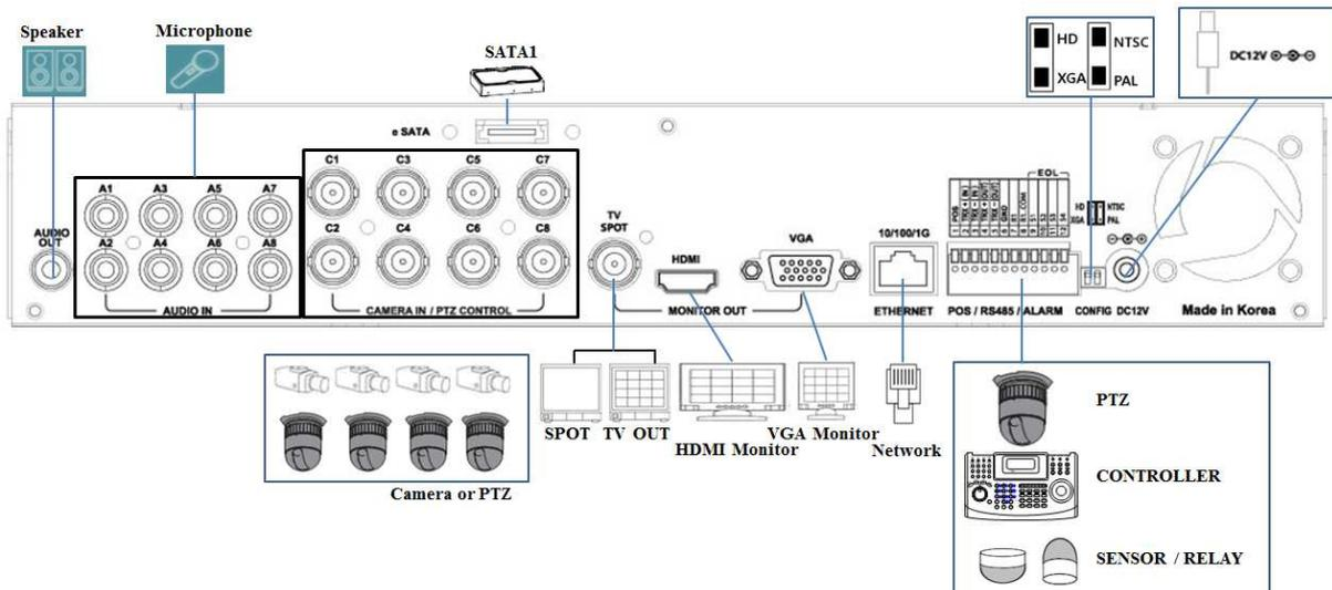
[Figure 2-5. MX-08A Basic Connection and Device Connection]
