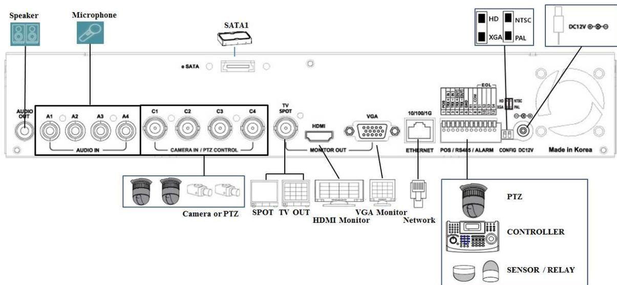
[Figure 2-4. MX-04A Basic Connection and Device Connection]
