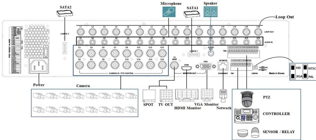
[Figure 2-1. MX-16PROA Basic Connection and Device Connection]
