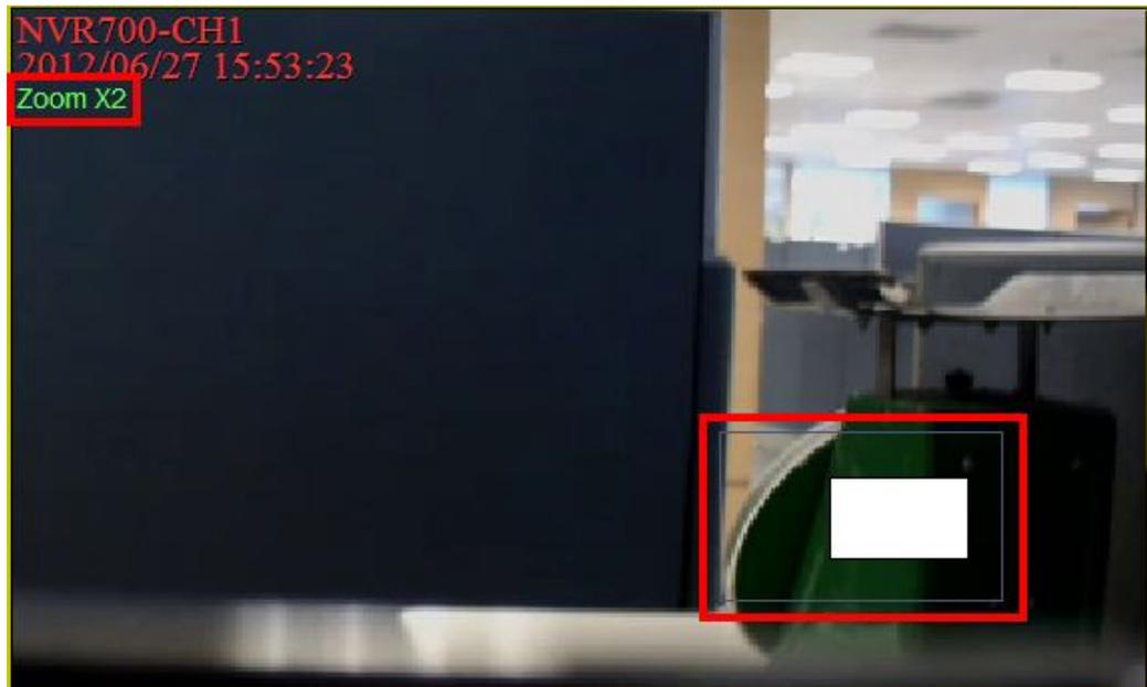
On the upper left-hand corner will show zoom-in multiple. The maximum multiple is X7. Also on the lower right-hand corner will show the position of current viewing area, shown as an inner white rectangle, comparing with the original screen, shown as an outer rectangle frame.
